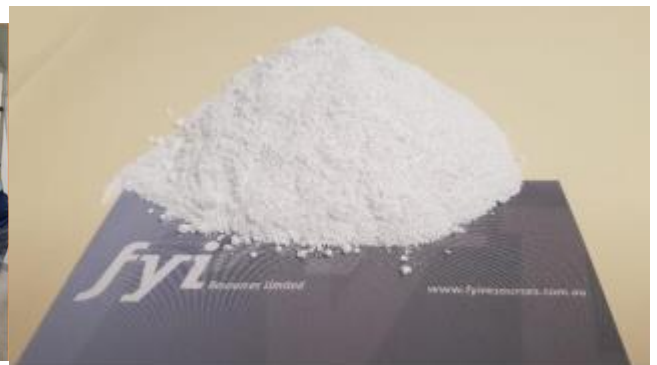
Figure 17: HPA produced from pilot plant
